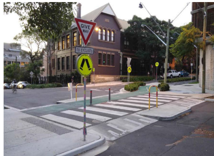
Separated pedestrian crossing (Source: Austroads, 2017)
