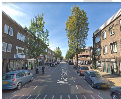
Path type: Mixed traffic – advisory bicycle lane Location: Utrecht, Netherlands Source: Google Street View, 2018
