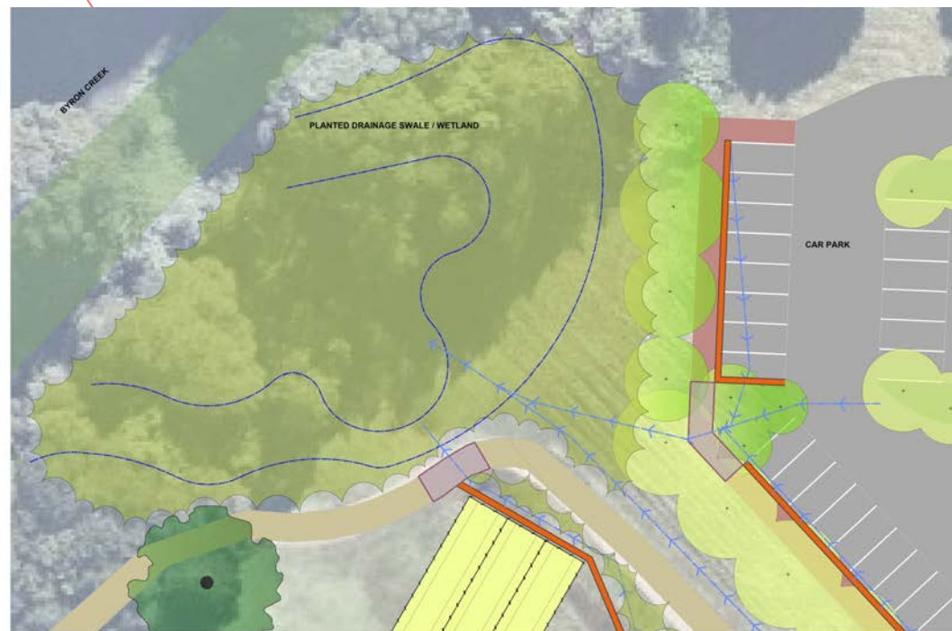
Figure 4. Northern carpark water sensitive urban design concept
