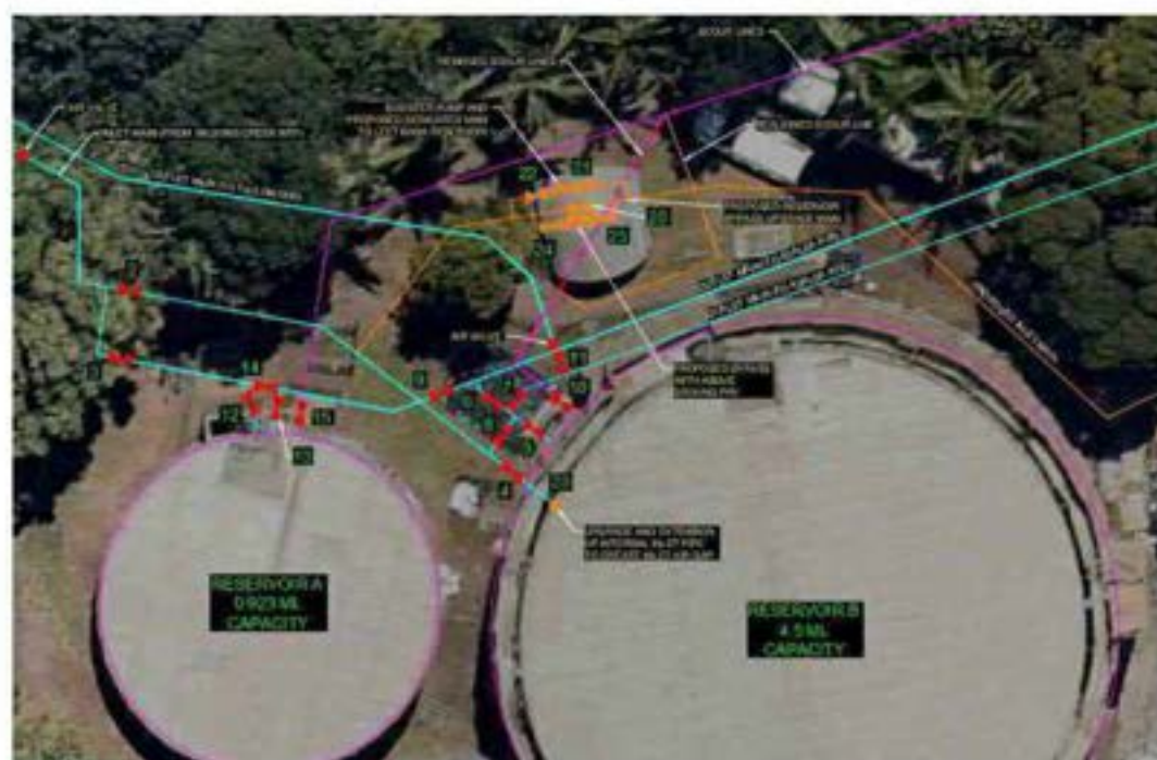
Figure 12 | Recommended Azalea Street Reservoir Bypass Arrangement
