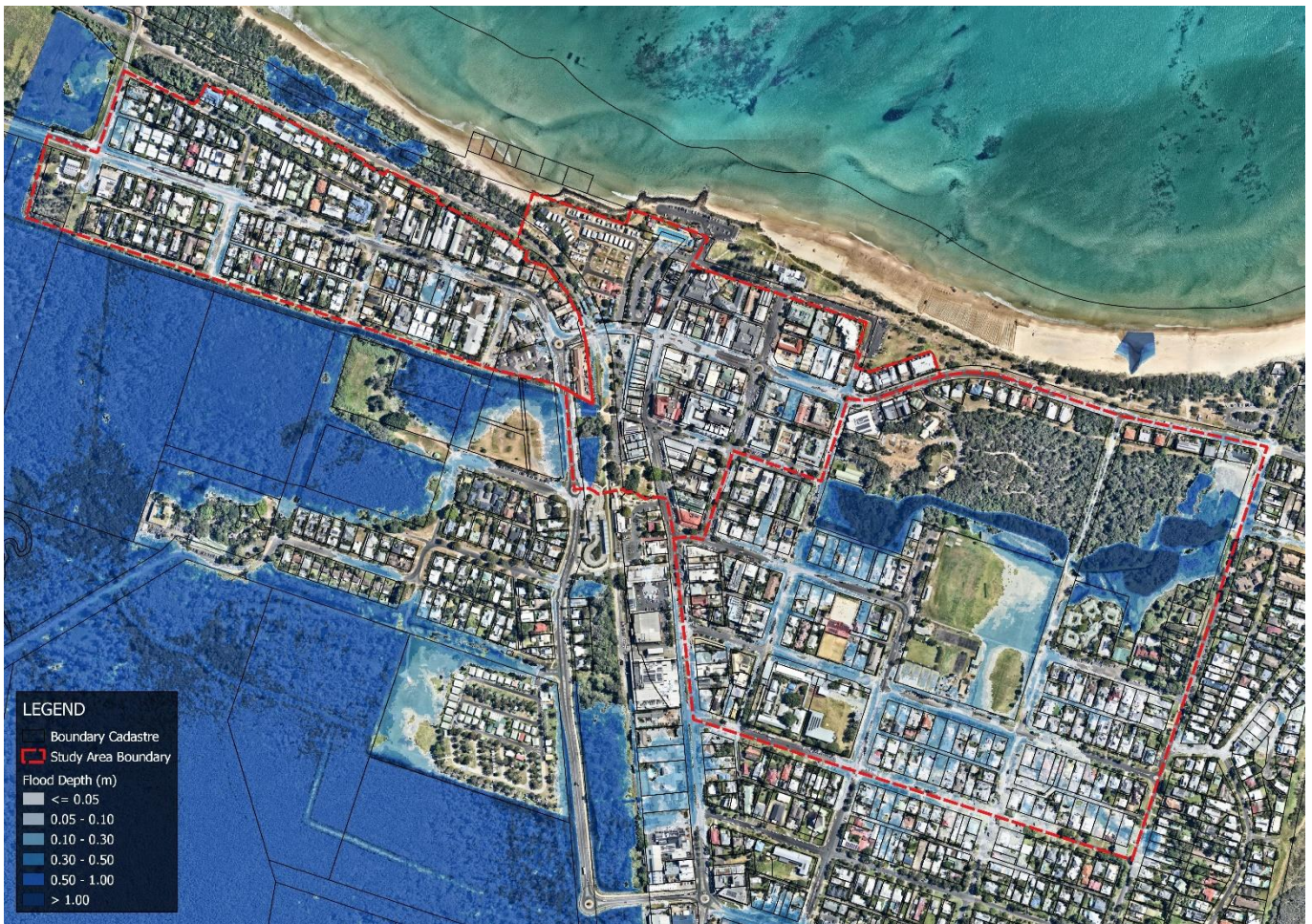
FIGURE 4.10: 10% AEP DESIGN UPGRADE SCENARIO FLOOD DEPTH
