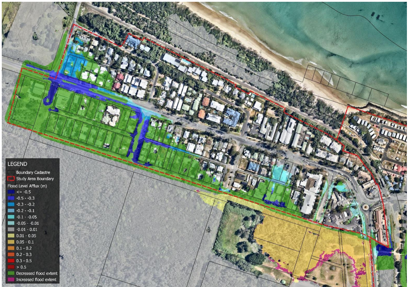
FIGURE 4.11: 10% AEP DESIGN UPGRADE SCENARIO FLOOD LEVEL AFFLUX
