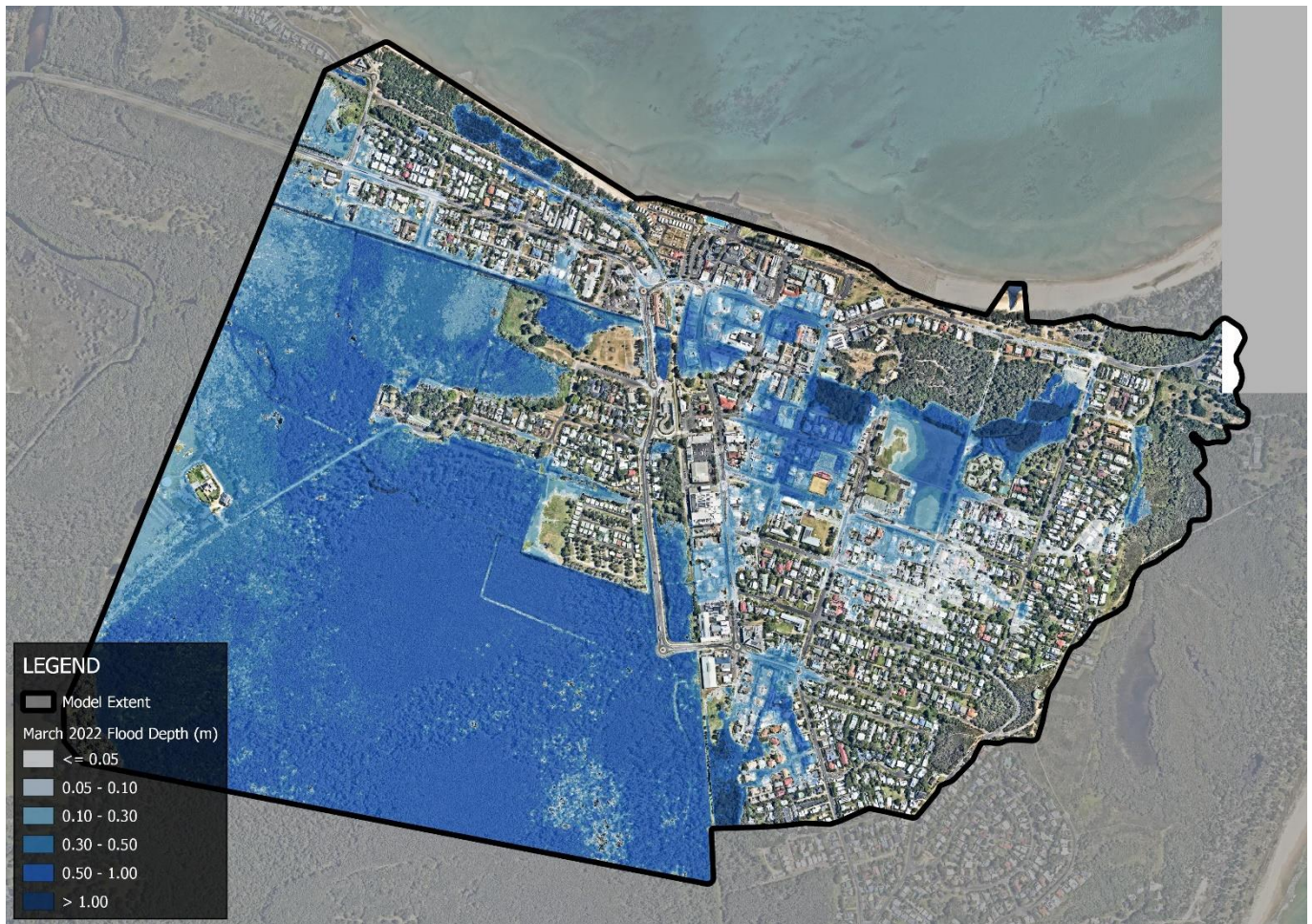
FIGURE 4.5: MARCH 2022 MODELLED FLOOD DEPTH
