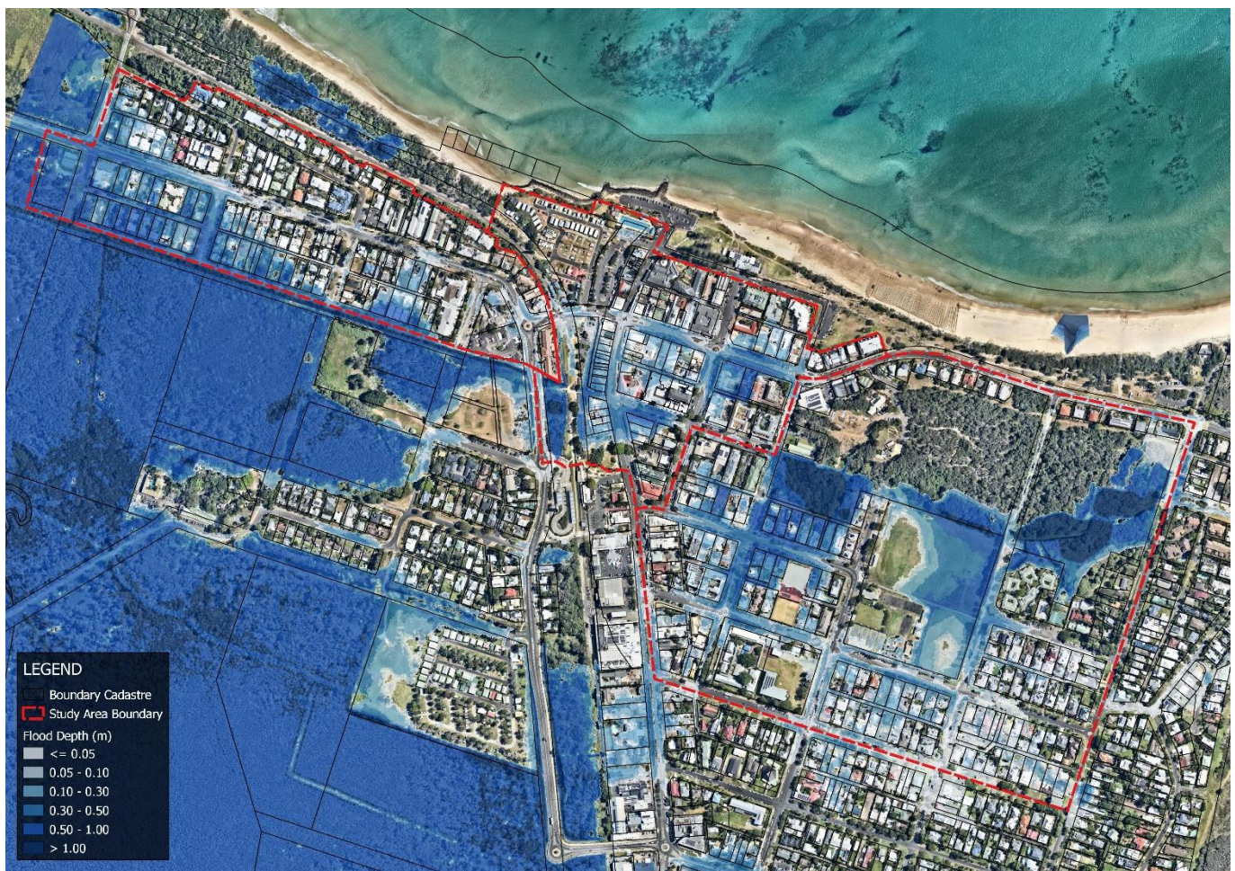
FIGURE 4.7: 10% AEP BASELINE SCENARIO FLOOD DEPTH
