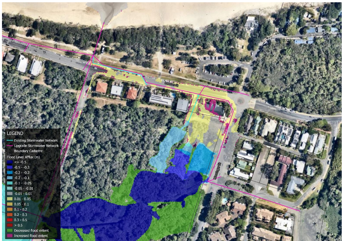
FIGURE 4.18: PROPOSED MASSINGER STREET TRUNK DRAINAGE 10% AEP FLOOD AFFLUX
