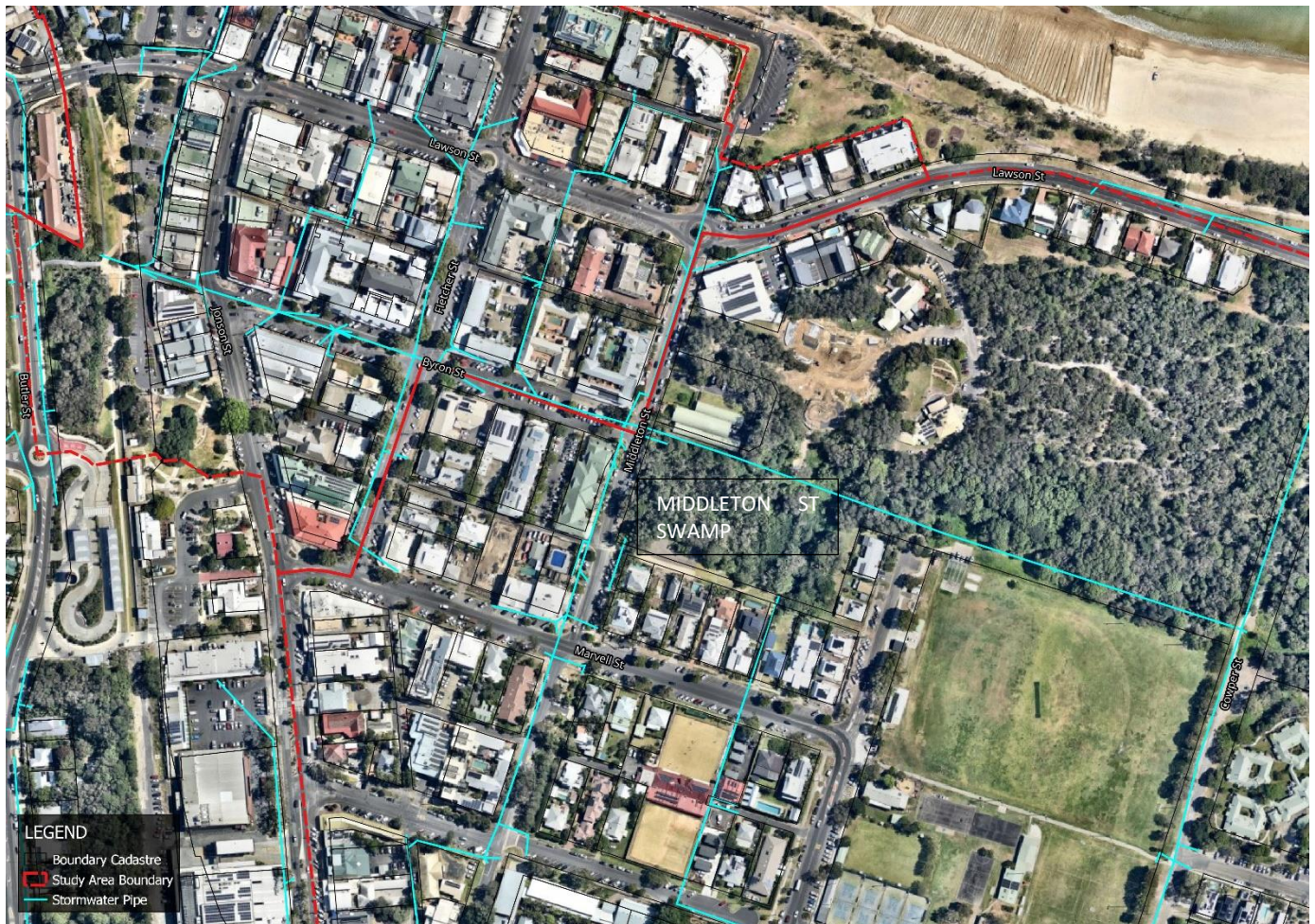
FIGURE 4.8: EXISTING SCENARIO PIPE NETWORK LAYOUT
