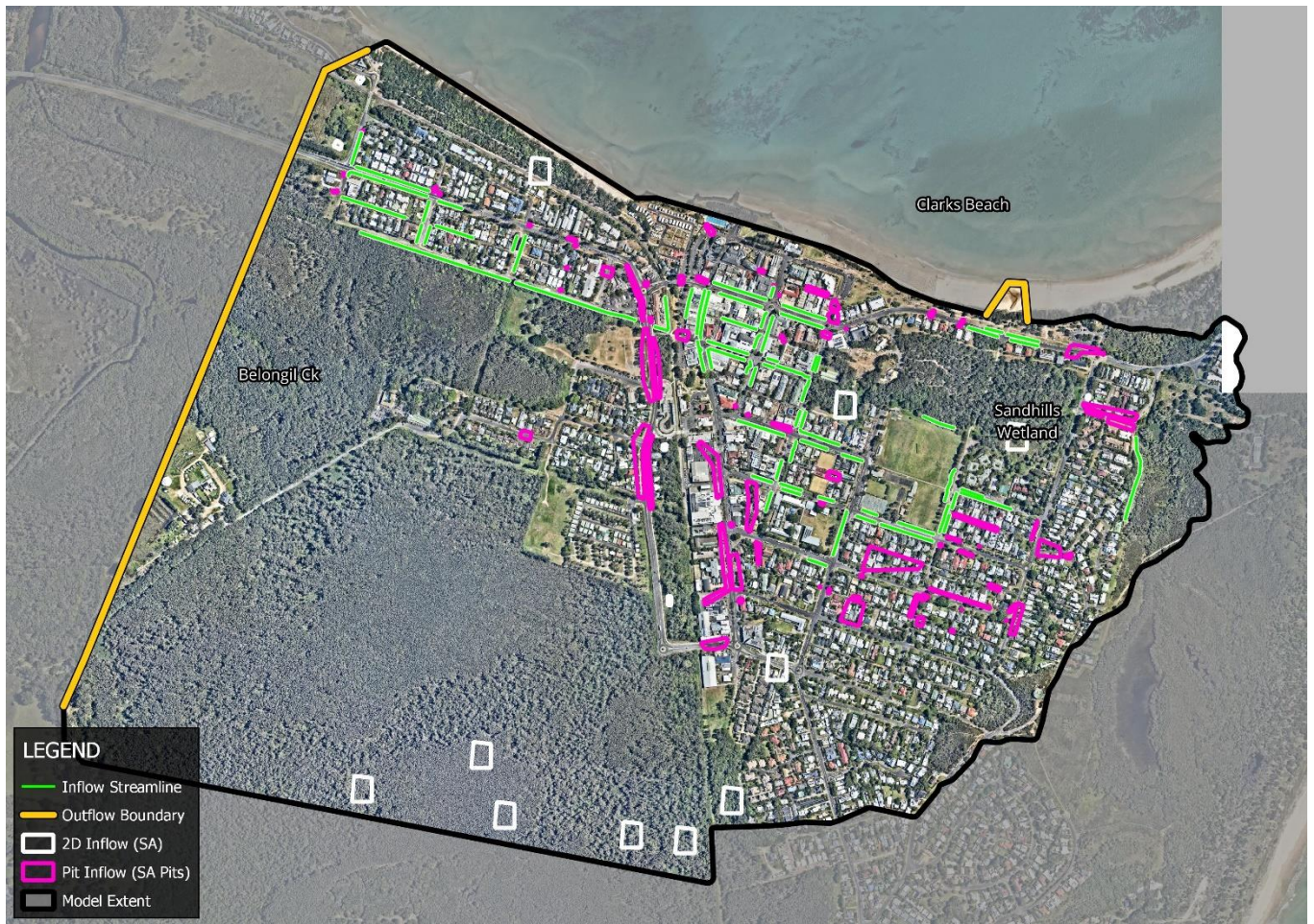
FIGURE 4.2: TUFLOW STORMWATER NETWORK AND BOUNDARIES
