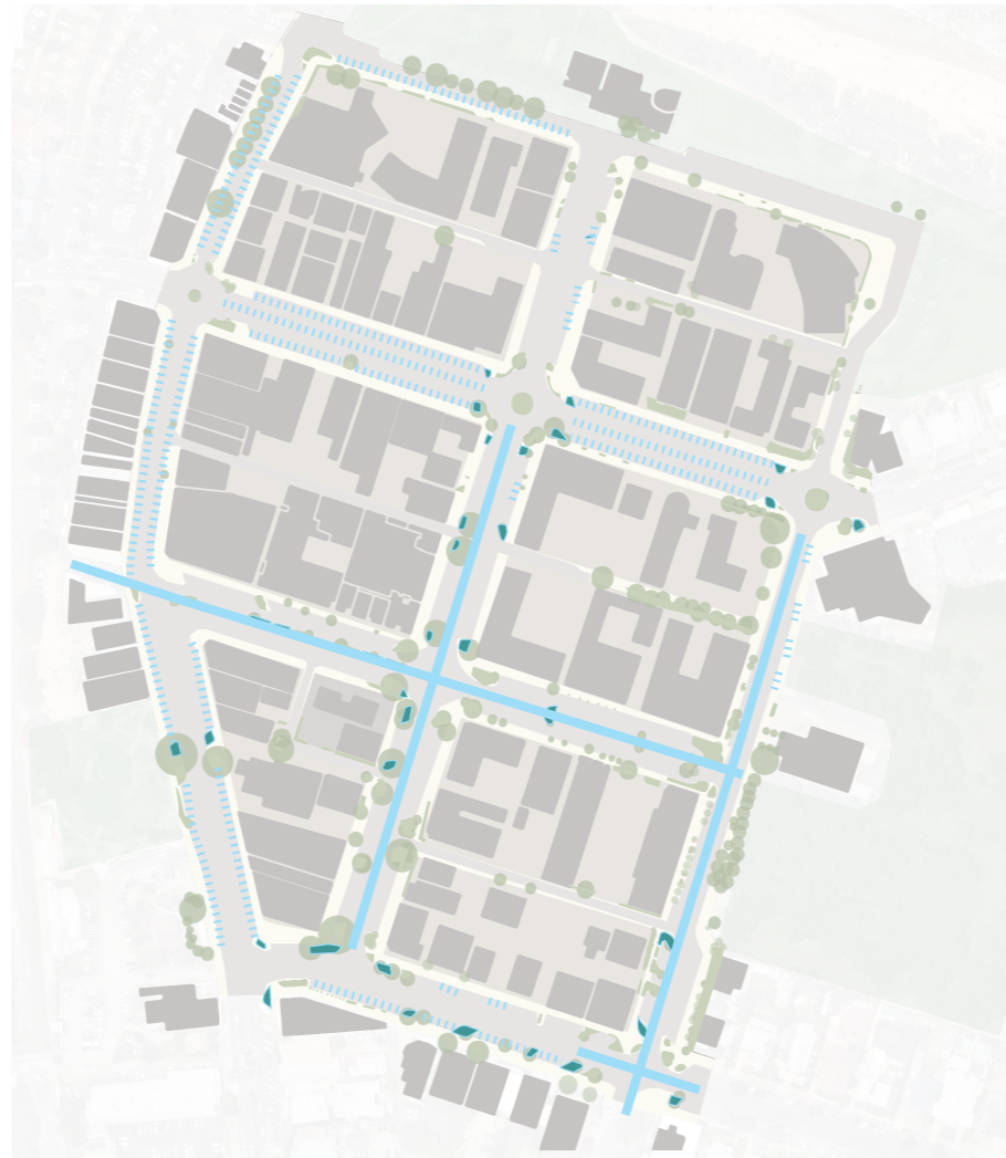
Tree grates implemented to allow full width pavements while storm-water is captured to water
