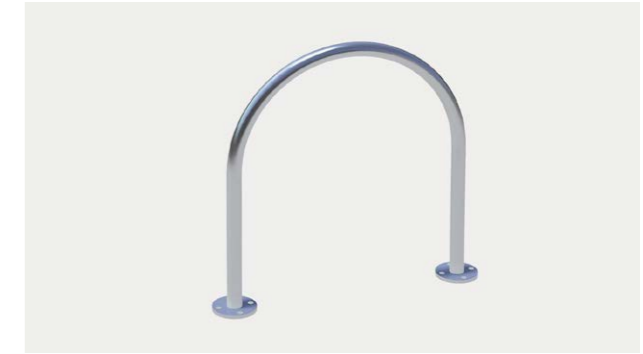
BICYCLE PARKING Name: Semi-Hoop Code: BST03 Dimensions: 845L x 120W x 850H Fixing: Surface mounted Material: Stainless 316 Finish: No.4 Finish (brushed) Supplier: Street Furniture Australia
