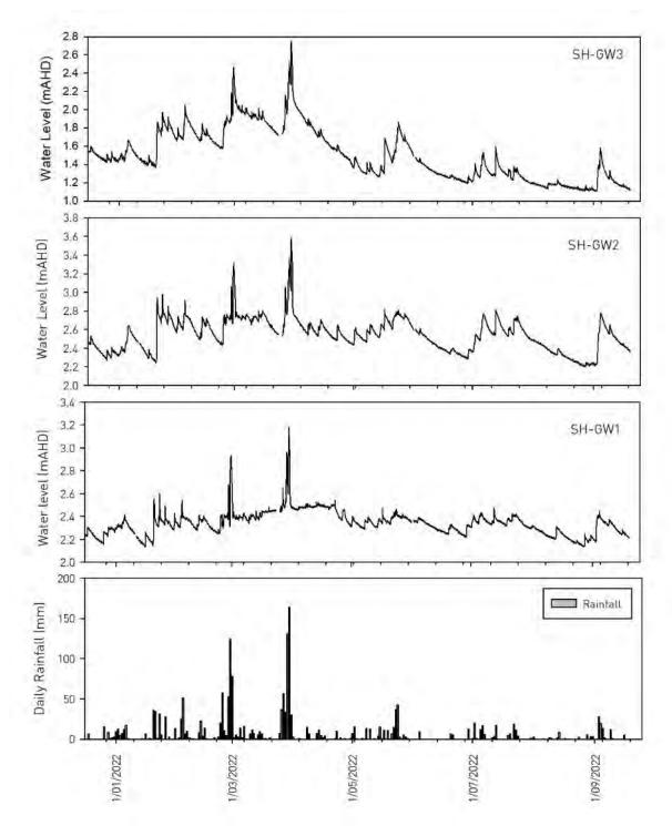
Figure 6 Groundwater monitoring data and rainfall for the Sandhill site January 2022 - October 2022.
