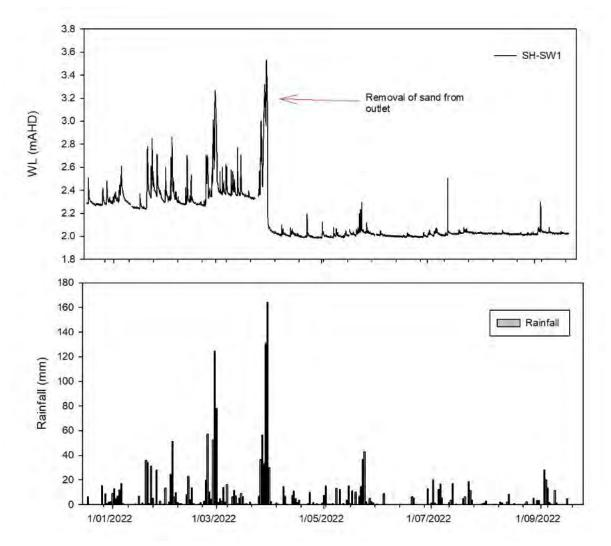
Figure 7 Surface water quality monitoring data and rainfall for the Sandhill site January 22 -October 22.
