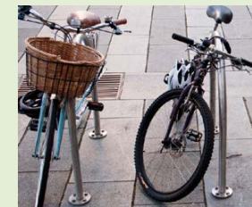
'SEMI HOOP' BIKE RACK [BST03] Material: 316 Stainless steel Finish: No.4 Finish (brushed) Size: 845 L 850 H 120 W Fixing: Surface or subsurface depending on surrounding surface Supplier: Street Furniture Australia
