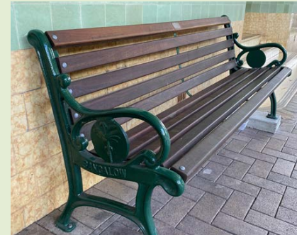
CUSTOM 'BANGALOW' COUNCIL SEAT Material: Recycled cast aluminium with hardwood timber slats Finish: powder coated / Cutek stain Colour: Heritage green Size: 1875 L 800 H 588 W Signage: Custom bangalow palm detail Fixing: Surface mounted Supplier: Landmark
