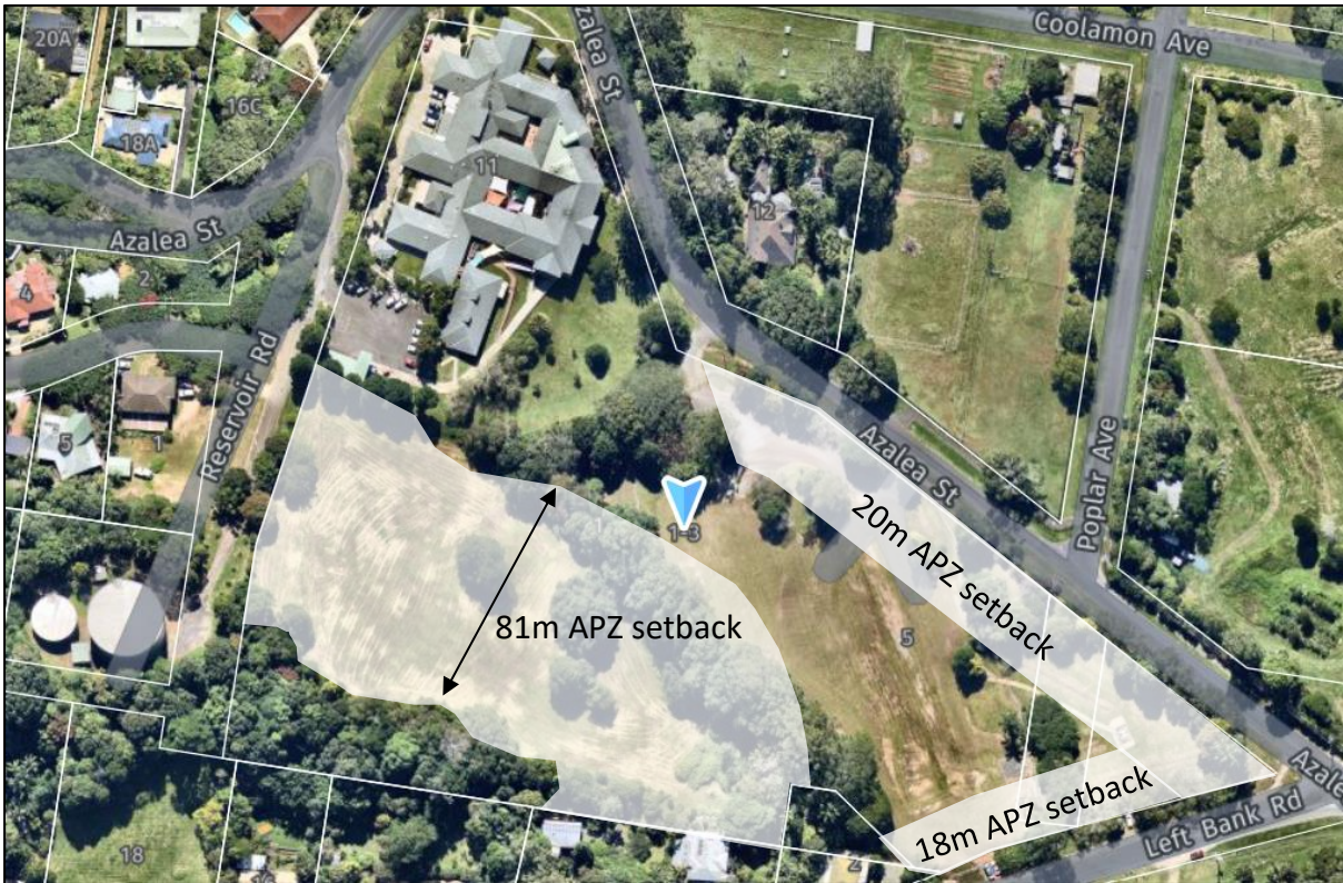
Figure 12: Preliminary asset protection zones residential SFPP – merit to reduce the APZs with future performance solution subject to NSW RFS concurrence.
