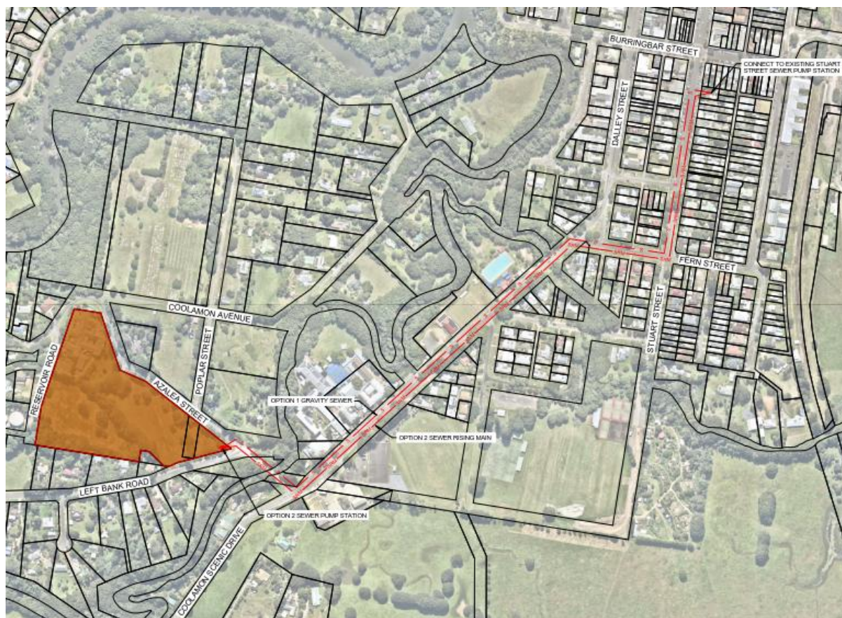
Figure 4-3 | Sewer Servicing Options
