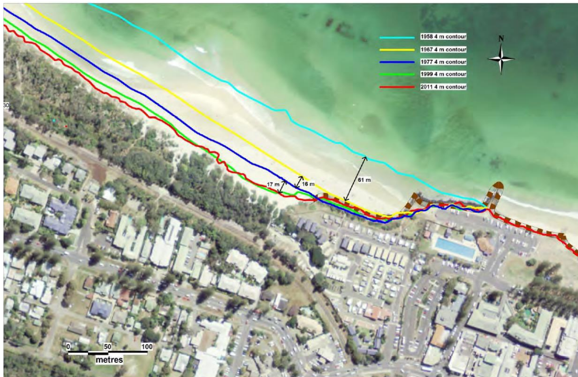
Figure 33: Historical analysis of position of the 4m depth contour downdrift from the JSPW using photogrammetry data (source: WorleyParsons, 2013).
