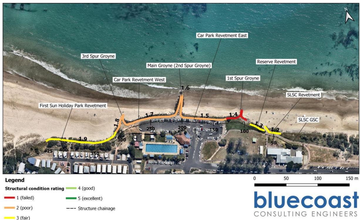
Figure 18: Structural condition rating for JSPW based on visual and drone inspection on 28 th October 2019.
