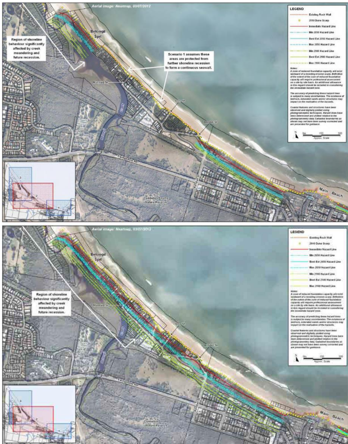
Figure 36: Coastal erosion hazard lines for areas downdrift of the JSPW (top) under 'Scenario 1' that coastal protection structures are maintained and (bottom) under 'Scenario 2' that coastal protection structures are removed (source: BMT WBM, 2013).
