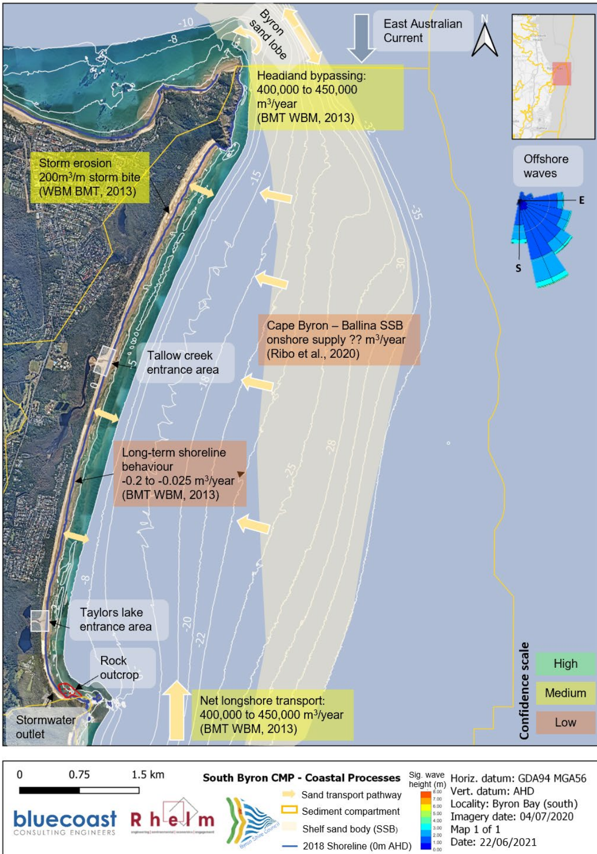
Figure E-2: Summary of the current coastal processes knowledge for Broken Head Beach/Tallow Beach Embayment
