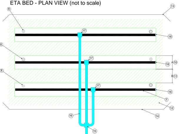
Component 7. 100 mm PVC pre-slotted pipe oriented and levelled to ensure even distribution of effluent
