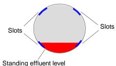
Component 13. Profile of downslope diversion diversion swale and drain.
