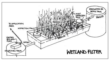
Typical reedbed wetland (includes septic tank and pump well)
