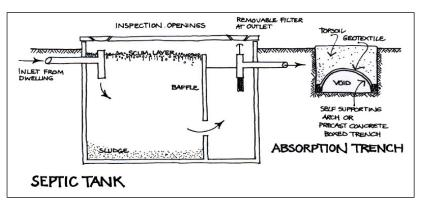
Side view of a septic tank and trench
