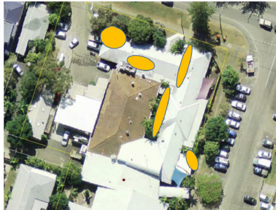
Figure 1 - 10-12 Shirley Street – areas of elevated radioactivity (above background levels) highlighted in yellow
