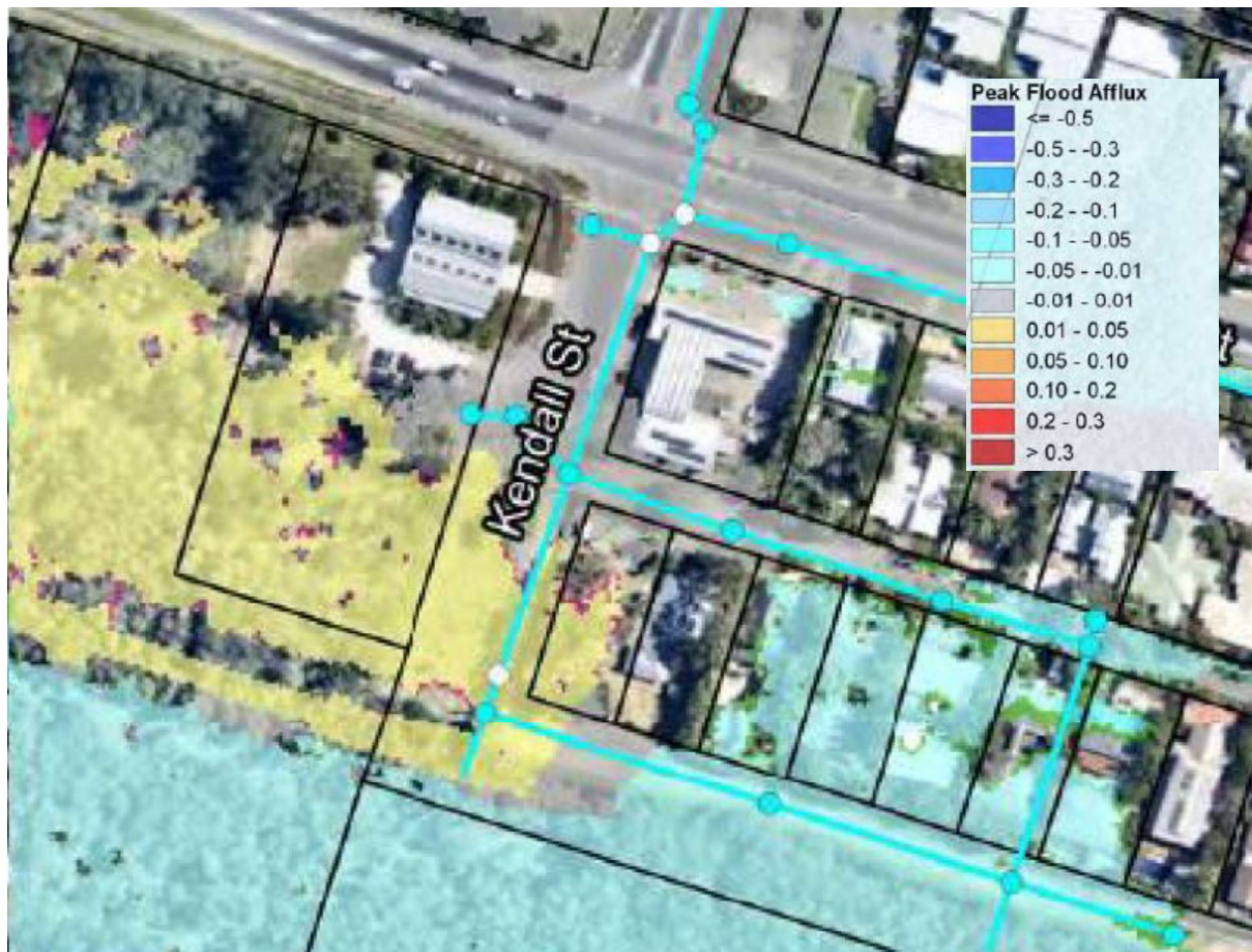
Figure 3-5 | Flood Afflux at Kendall Street from the proposed gravity drainage system upgrades
