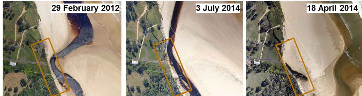
Figure 97: Aerial photographs showing progressive erosion of northern entrance embankment at Belongil Creek prior to geotextile container revetment construction in 2015.
