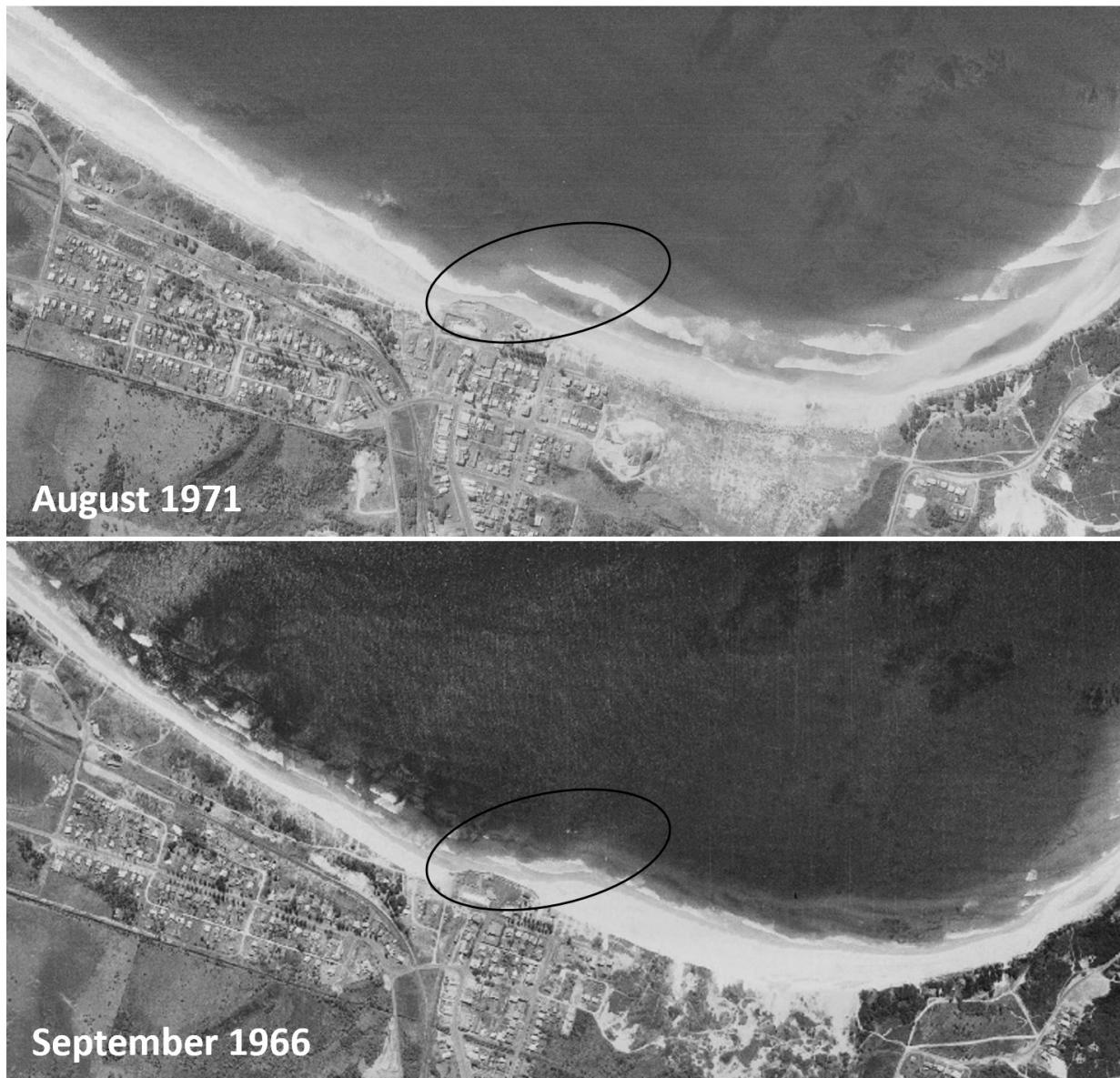
Figure 58: Two historical aerial images highlighting the bulge of sand in the lee of Middle Reef wave shadow and nearby JSPW.
