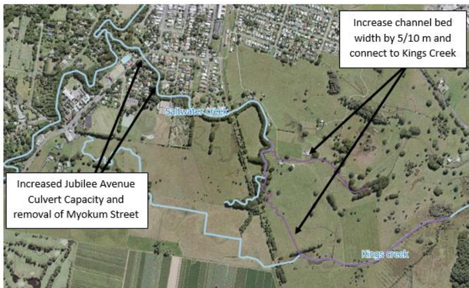
Diagram 43: Option SC2b - Removal of Myokum Street embankment, increased Jubilee Avenue culvert capacity and increased capacity
