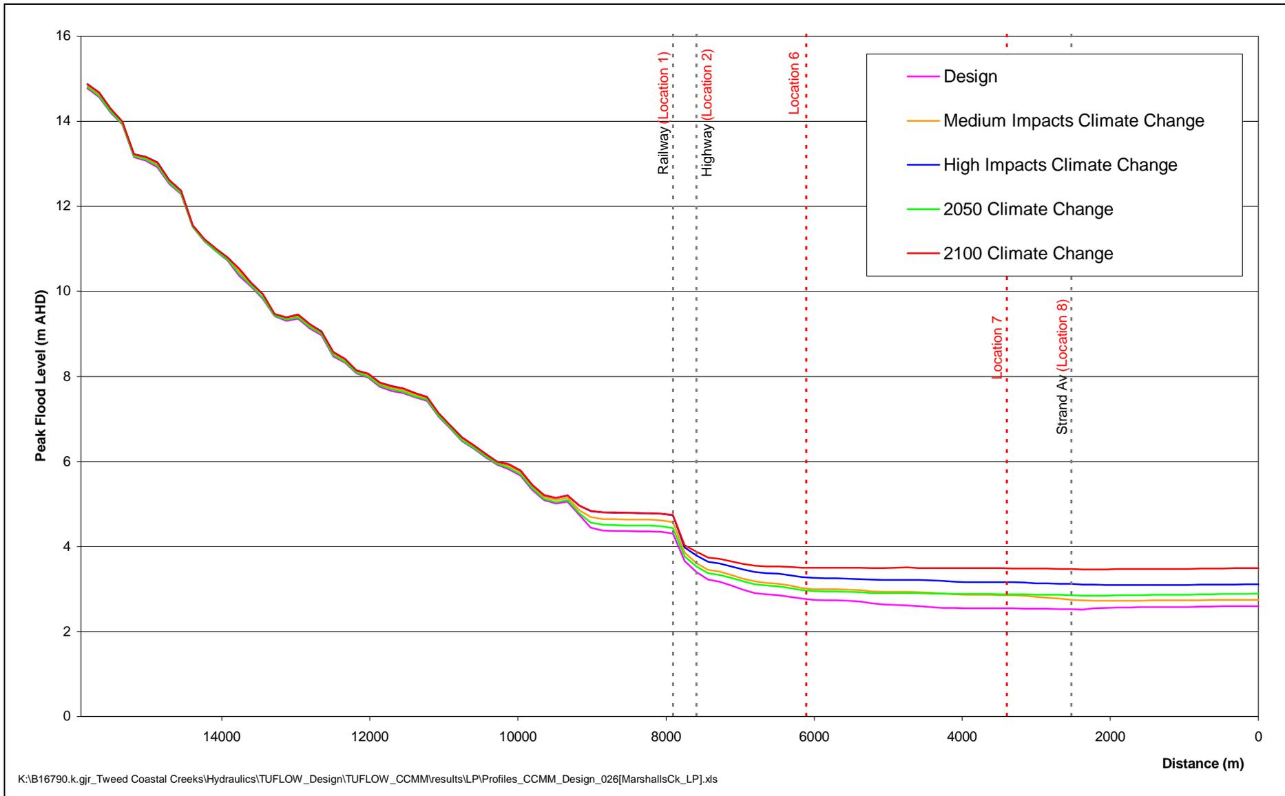
Figure 3-11 100 Year ARI Peak Flood Levels Marshalls Creek Long Section
