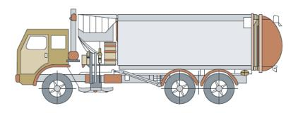
This is the most commonly used vehicle for domestic garbage and recycling collections. It is only suitable for collecting MGBs up to 360 litres in size.
