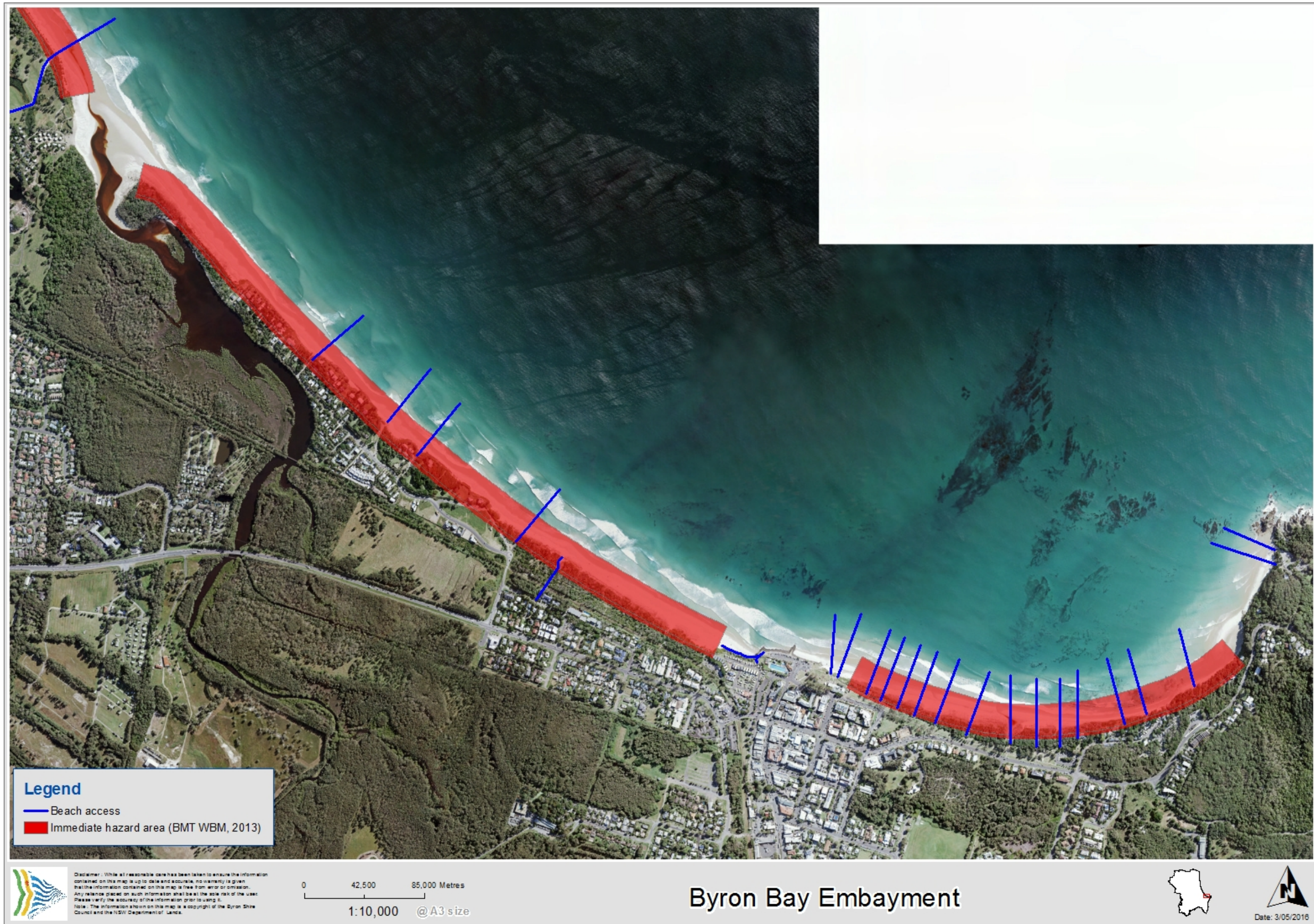
Figure 4-3 Byron Bay Embayment, immediate hazard area includes 11m allowance for the zone of reduced foundation capacity (2015 aerial photography).
