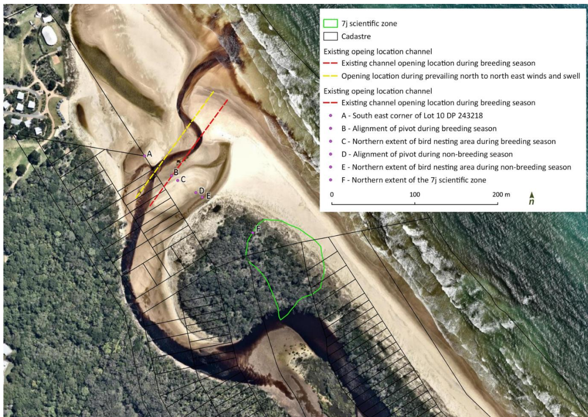
Figure 6. The proposed opening arrangements for Belongil Creek estuary entrance
