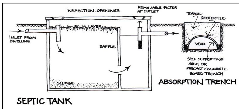
Side view of a septic tank and trench
